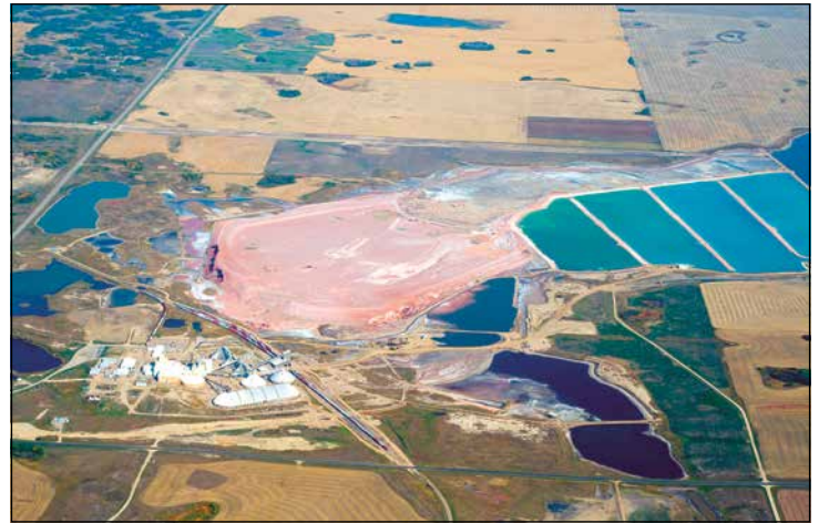
Monitoring surface mine infrastructure such as buildings, headframes, mill and processing, as well as tailings containment areas and waste piles ensures compliance with environmental safeguards and corporate social responsibility. Above, the blue rectangular water features are tailing containment areas, the pink area is a large waste pile. InSAR can detect even slight changes that could jeopardize the stability of both areas.
